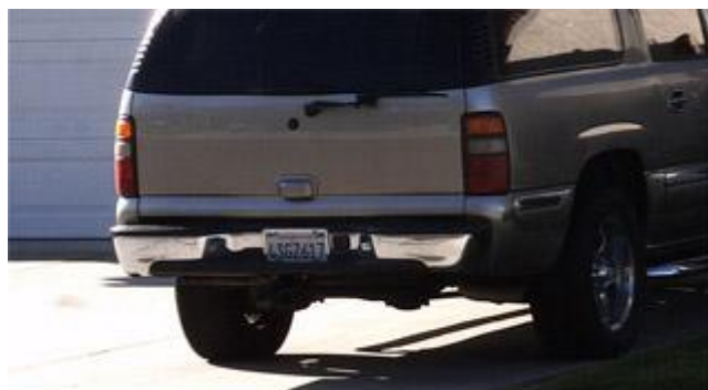
"License Plate," 1280 x 720p / 60fps / Lens: C-mount, 50mm, f/16/Daylight. Car ~ 50m away.
